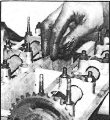
Measuring the valve clearances. With all new valves, seats etc. start with a nominal 80 thou. shim and work up.
