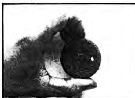
Block core plugs are automatically changed by us on every rebuild. Only a build up of rust and Bars Leak prevented this rear plug from leaking.
