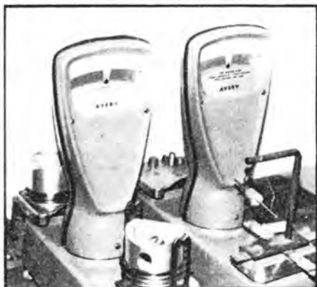
The piston assemblies being balanced. The other set of scales are used in conjunction with the first set for end to end balancing of the con rods.
