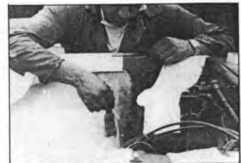
Laminating inside the engine bay join. 1oz (300gm) mat is being used.
