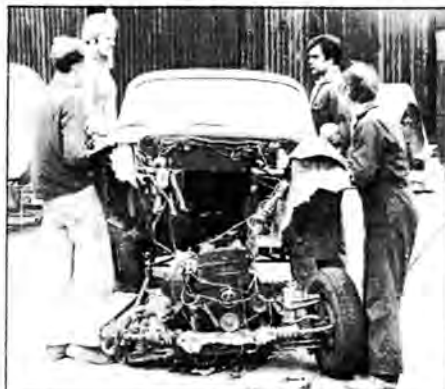
Lifting the body clear, the back end is heavier even when there is a complete body. Weak ones take the front.
