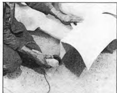
True-ing the new section up with the grinderette.
