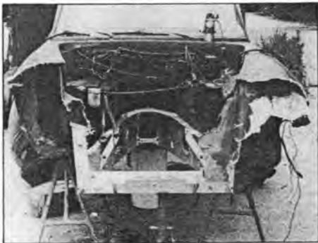
The new chassis is offered up into the body recess and held firmly in its correct position. (Don't forget that the felt must be in place).
