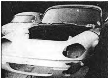
Offering the new section up using the chassis as a platform.
