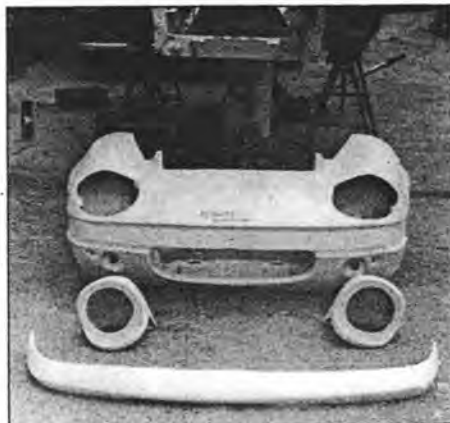
The new body section and headlight pods and bumper. All come from the factory in primer-surfacer.
