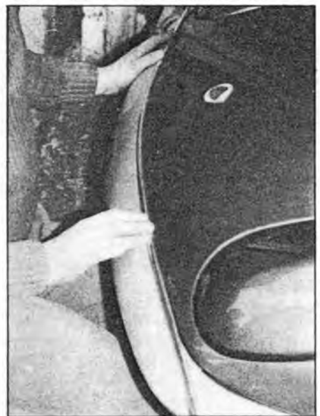
Fitting the front bumper strip; a hair dryer is a must for warming up the strip to bend it into place around the corners.
