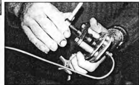
We do all our own brake lines. These brake flaring tools are fairly inexpensive and worth their weight in gold.
