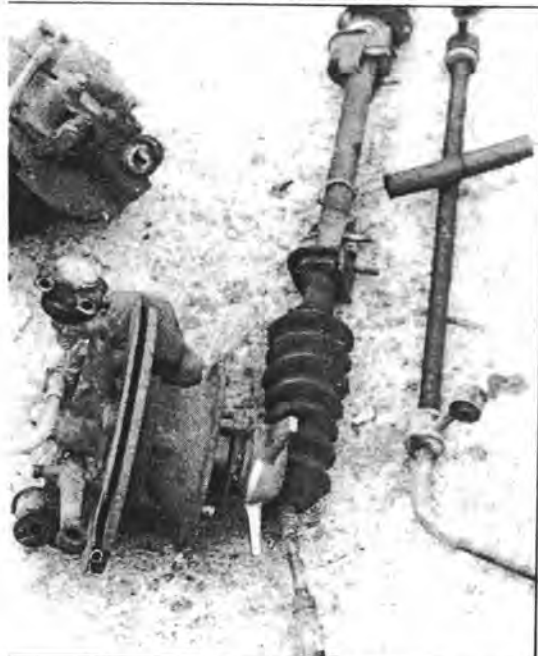
Part of the front running gear; rack is being replaced as a whole assembly. Note that the anti roll bar bushes have swollen with oil and age — these will be renewed.
