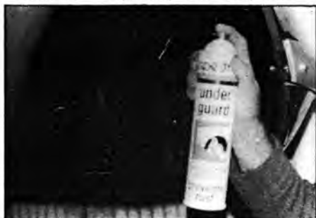
Making a neat underside using an aerosol under-seal spray. This also serves to stop stones piercing the underside of the wing, eventually causing gel cracks (little stars) on the top surface.
