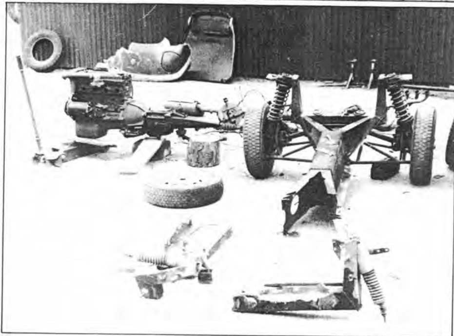
Part of the front running gear; rack is being replaced as a whole assembly. Note that the anti roll bar bushes have swollen with oil and age — these will be renewed.
