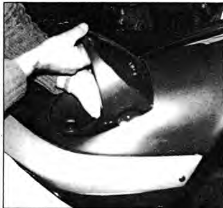
Very carefully bolting in the headlamp pod so as not to damage the new paint surface.
