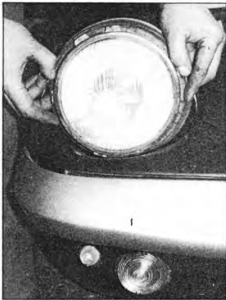
Fitting the headlight unit — after the vacuum tanks, etc. have been fitted.
