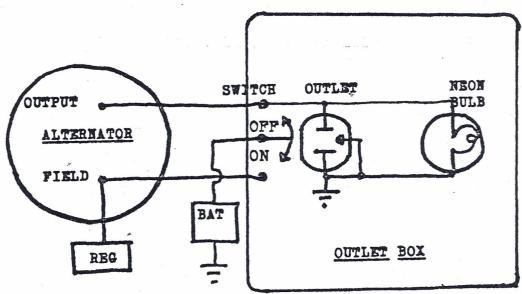
Note: Neon bulb lights up when 110v is available but remains off when using system for welding.
