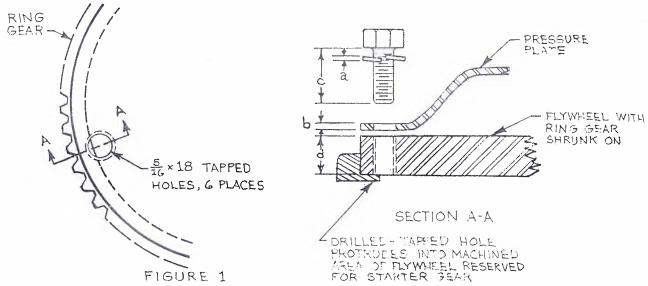
Another item to be aware of is that 110-tooth ring gears no longer come with a bevel on each side of the teeth, forcing the rebuilder to decide which style starter he will use and to install the gear accordingly.
