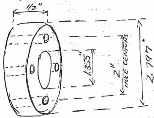
The fan and spacer must be drilled to mate with the four holes in the hub. The old bolts should be replaced with new ones 1/4" longer and these should be treated with lok-tite to preclude their loosening due to vibration.
